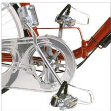
014 Fixed Footrest Left 015 Fixed Footrest Right For individuals with rigid leg or fixed knee joint
