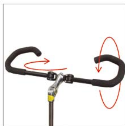
093 Multiposition handlebar The end and the middle section are adjustable separately which allows excellent adjustments for the individual sitting position. Thus also asymmetric adjustments are possible.
