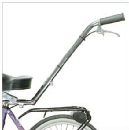
238 Guide Rod with Brake Allows caregiver to control brake
